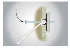
Snap off strap flush with collar. Insert the bolt through the fixture into the anchor and tighten securely.
