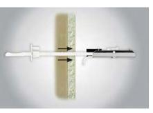
Insert the FlipToggle into the drilled hole. When the head is fully inserted, pull the strap to flip the toggle flat against the back of the wall.
