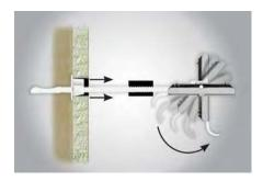
3.Push the collar into the drilled hole until the cap is flush with the wall. Hold the cap against the wall while pulling the strap toward you until it feels reasonably tight.
