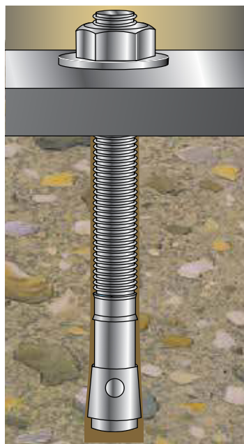
TRUBOLT® WEDGE ANCHOR
